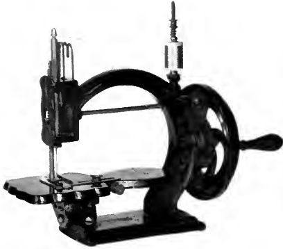
Figure 90.—GRANT BROTHERS SEWING MACHINE, 1867. This machine was one of several styles that utilized Raymond's 1861 patented chainstitch method. This machine, however, used an under feed rather than a top feed.
